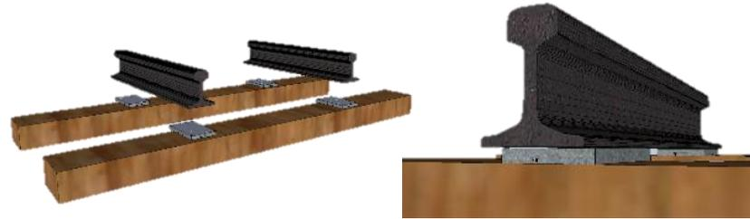
Due to the high pressure applied by the train, the piezoelectric material cannot be directly placed as it could break. So that they have to suffer less, we have designed a module composed by four piezoelectric ceramics and by four other shock absorbers.
